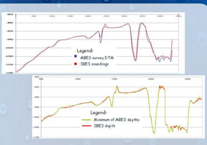
The beam footprint was modelized using a disk with a radius defined as a function of the depth. As attempted, the SBES soundings mainly vary according to the shoalest depth belonging to its footprint. As mentioned by Mark and smith in [9], the SBES uncertainty is also a function of the
