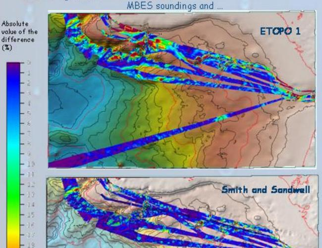
A bathymetric profile of 100km length allows comparing the three DTMs in terms of wavelengths. On the graphic depicting the signal energy for different wavelengths, we notice a slope break at 30 km for the ETOPO1 grid while the slope break of the Smith and Sandwell model occurs at approximately 10 km. This result observed on the selected bathymetric profile is confirmed by the coherency graph.
