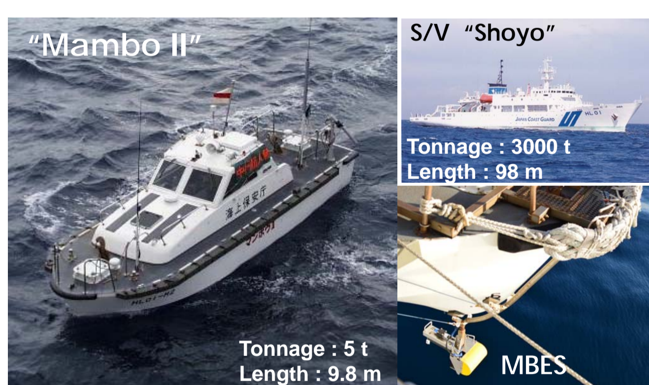
Fig. 10 Autonomous survey boat "Manbo II" (left), her mother vessel "Shoyo" (upper right), and a MBES (R2sonic2022) mounted on the Manbo II (lower right). Manbo II was designed for survey of active submarine volcanoes and was commissioned in 1998.
